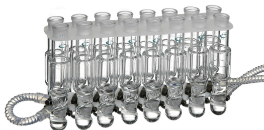
Figure 2: Array of Chemspeed 16 x 13 mL glass reactors used in the study.
