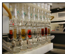
Picture 1: Reactions performed on a 1 mL scale in an array of 2 mL reactors
