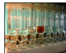
Picture 2: Automated liquid / liquid extraction carried out in the 13 mL reactors arrays
