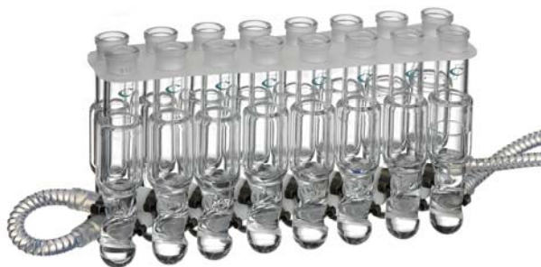
Figure 3. An array of 16 x 13 mL double jacketed glass reactors for use on the Chemspeed synthesiser.
