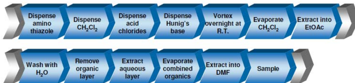
Figure 2. A typical amide coupling reaction workflow on the SLTII.
